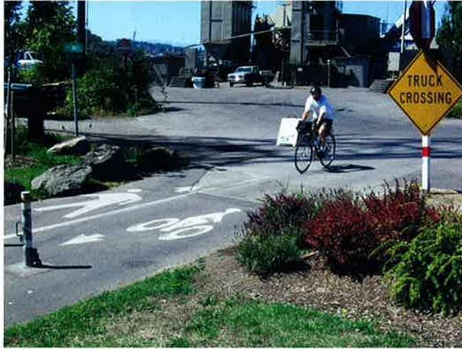
Signage where a multi-use trail crosses through an industrial route alerts cyclists that freight traffic is to be expected
